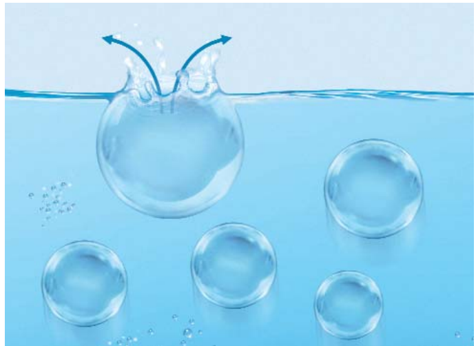
Figure 1: Rise and bursting of air bubbles in a surfactant-free liquid
