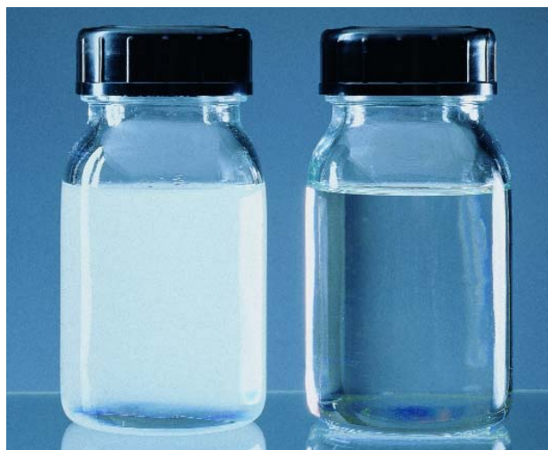
Figure 6: Clear coating containing silicone oil (left) and polyether polysiloxane copolymer (right)
