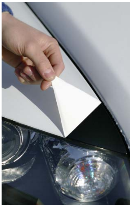
Figure 5: Release effect of transport protection films
