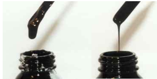
Figure 1: Resin containing carbon black grinds without and with additional use of a wetting and dispersing additive
