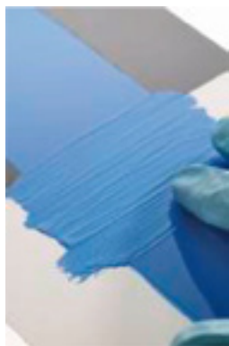
Figure 7: Rub-out test shows colour stability of a mixture of pigments
