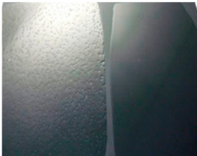
Figure 8: Removal of contamination craters (left: without; right: with substrate wetting additive)
