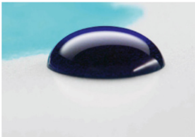
Figure 6: Contact angle showing good rewettability
