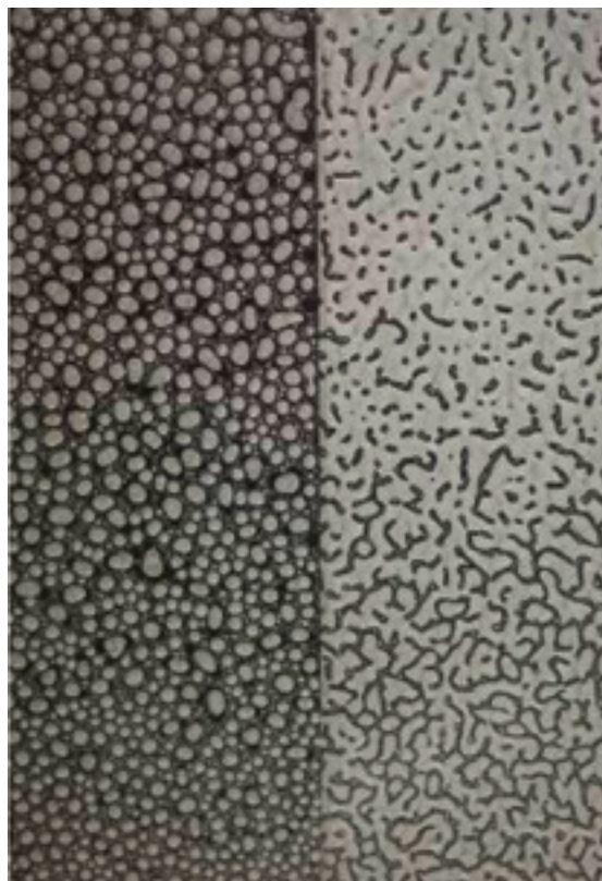
Figure 4: Substrate wetting by a silver paint on a dark background, wedge application (left: without; right: with substrate wetting additive)
